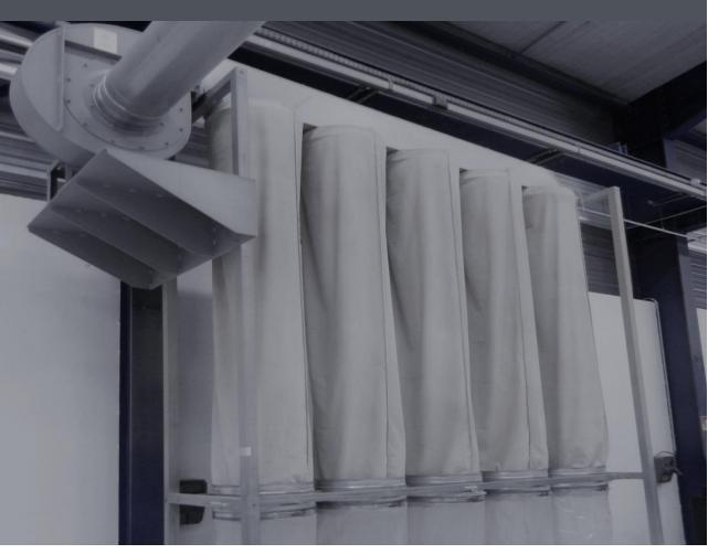
Processing residues and particles are separated from the material by aspiration all through the process.
